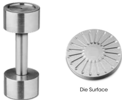
Torque Calibration Standard
