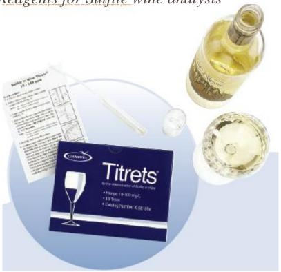
Range: 10-100 ppm as SO<sub>2</sub> MDL: 10 ppm / Method: Ripper
