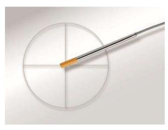
The Razor detector works in photovoltaic mode, without any bias voltage. Due to the ionizing effect of radiation, electron-hole pairs are created in silicon. The signal is mostly generated by electrons which, after freely diffusing through the crystal, reach the n-p junction region and are swept by the built-in electric field of the depleted region. Electrons of pair directly generated inside the depleted region provide a minor contribution to signal as well.
