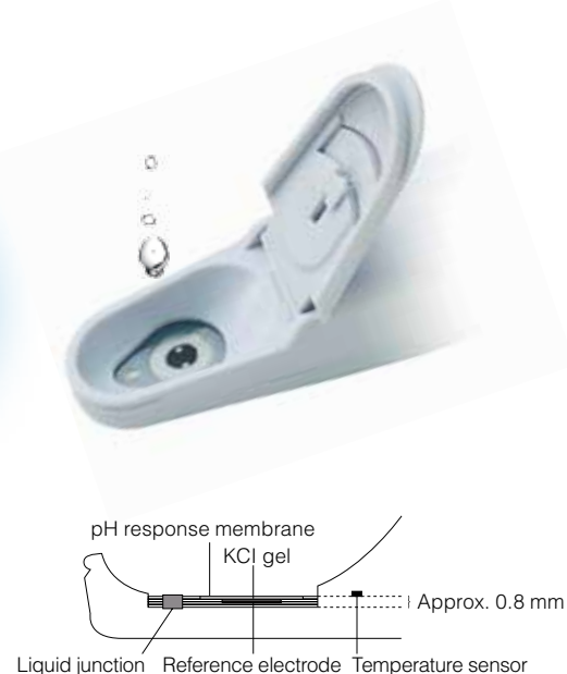
● Sectional drawing of tip of Flat sensor.
