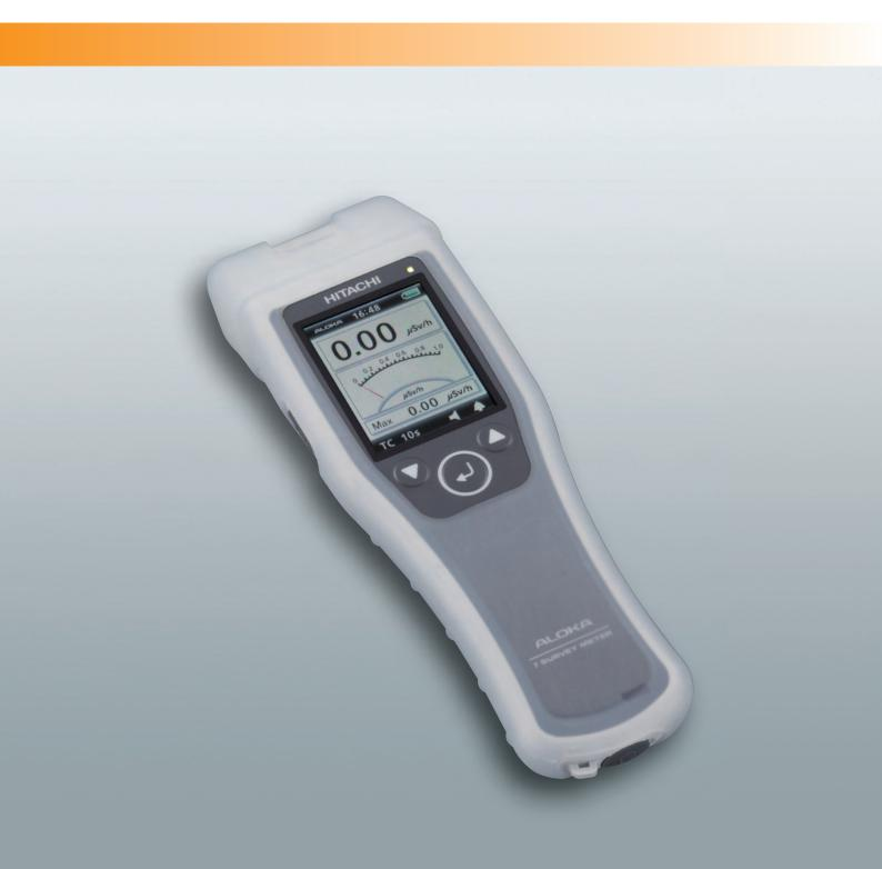
PDR-303 is a well-designed Gamma survey meter for ambient dose rate measurement with a comfortably compact shape. Semiconductor detector with the reasonable water proof (splash proof) structure enables comfortable measurement for any user. TFT color LCD assists users to read the value, and sufficient alarm features (display and sound) inform users when the dose rate exceeds the preset level.
