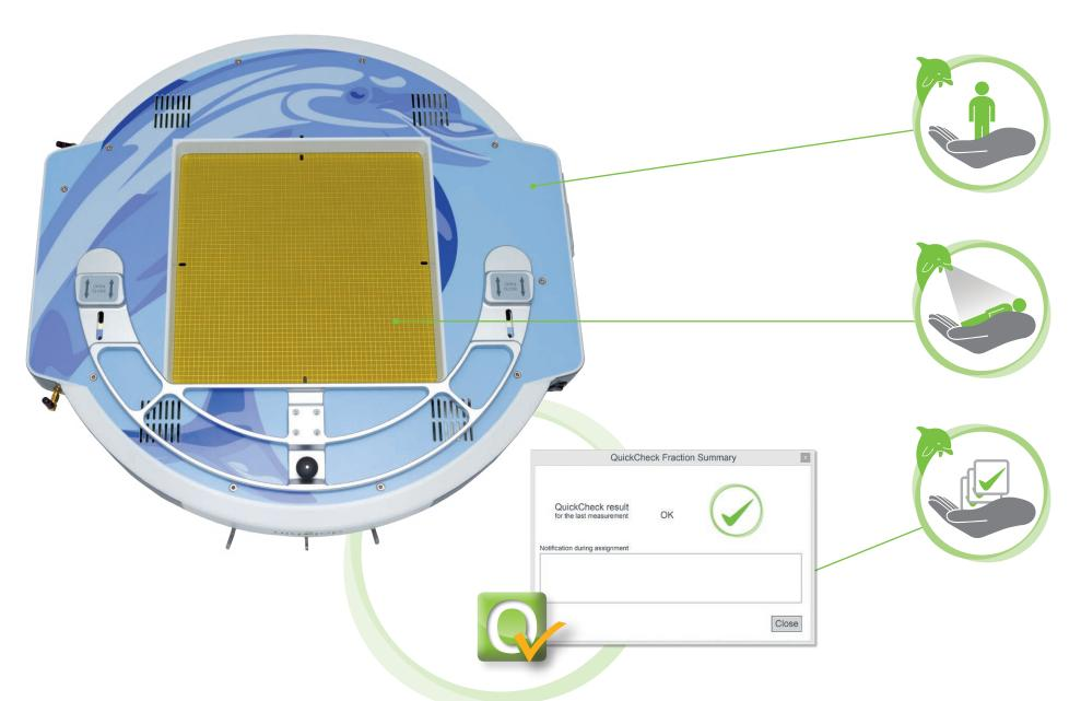
The Transmission Detector will offer an ultimate end-to-end test to independently verify any treatment technique (including complex treatments such as static IMRT/VMAT) and to visualize dosimetric outcome.
